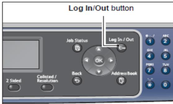
2. Enter passcode using the numeric keypad and press **OK** button
