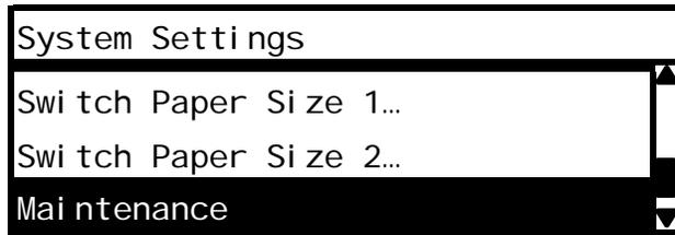
5. Enter "950807" using the numeric keypad on **Maintenance** screen and press **Start** button
