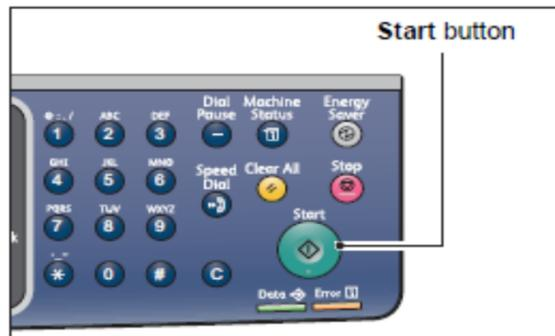
6. Press **Start** button if the Drum Cartridge has been replaced with a new unit or press **Clear All** to cancel this action
