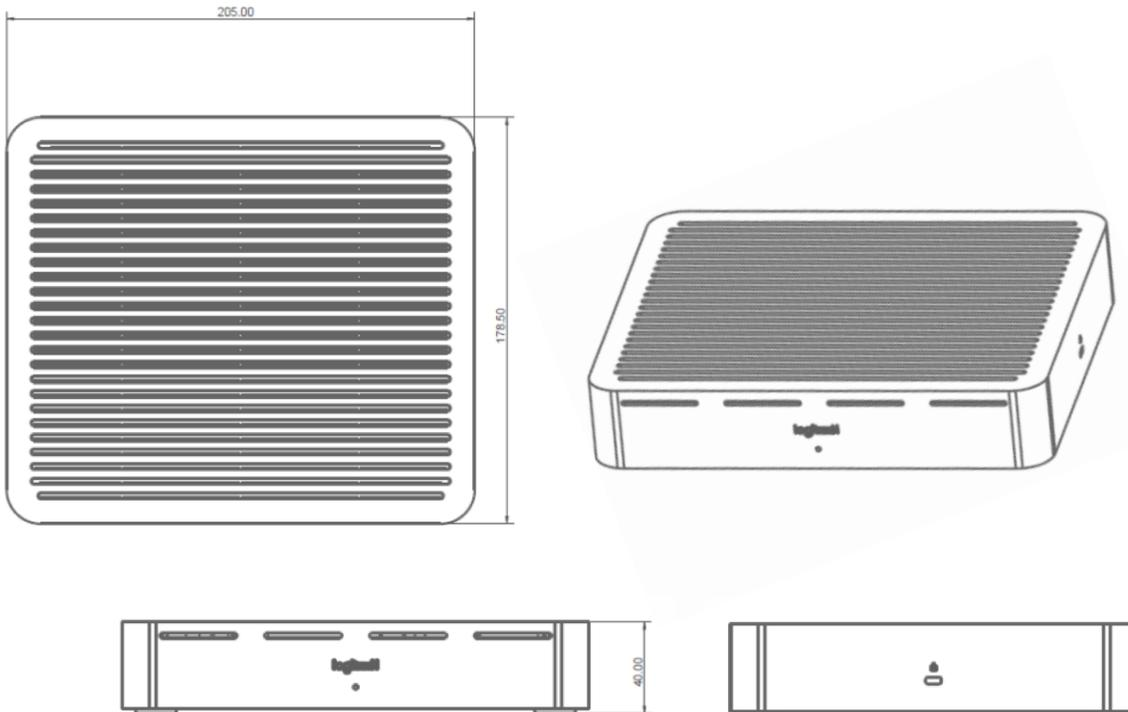
d. MIC PODS: Each Mic Pod has an approximate pickup diameter of 15'/4.6m. The microphones can be daisy chained or connected in a trunk/branch configuration using the optional Mic Pod Hub described below. Rally supports up to seven (7) Mic Pods.
