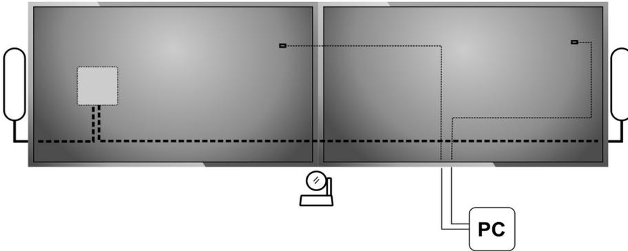
iii. Connect the USB C cable between the camera and Display Hub. The camera draws more power than normally available from an USB port and so must be connected to the Display Hub. Note, the camera can optionally be mounted upside down and an internal sensor will automatically invert the image and remote control function. The camera must be power cycled when mounting upside down.
