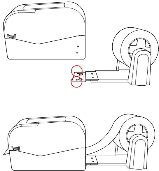
3. Insert a 3" (76.2 mm) Label Spindle into a paper roll. Then, install it on the External Paper Roll Mount.
