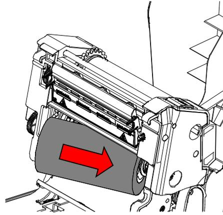
8. Thread the ribbon through the Print Head and adhere the leader of the ribbon onto the Ribbon Rewind Paper Core.
