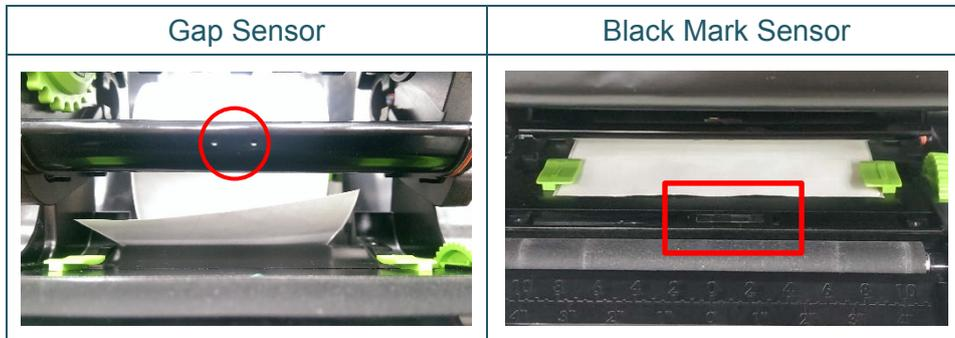
The transmissive/gap sensor detects the beginning of the label and feeds the label to the correct position.
