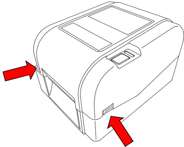
2. Push up the lock switch to unlock the Roll Guides.
