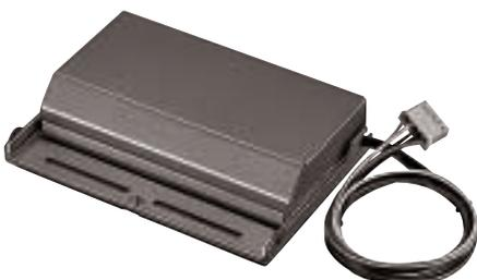
The AU-100 series detects the position of the cutter blade by means of a mechanical contact and controls the rotating direction of the motor. This allows the AU-100/AU-110 to achieve both partial and full cutting of paper.
